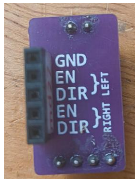
Motor driver component. See left and right EN and DIR pins.
