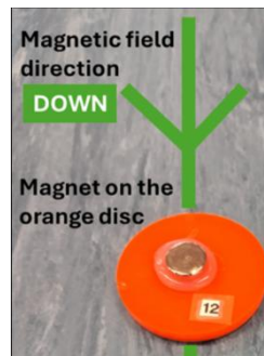
Magnet that will be placed inside the rock
